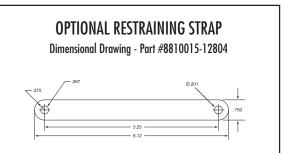
\*Please note, mounts are not inherently fail-safe. They may require the use of a suitable restraining device.
